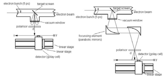
Figure 4: Set-up A (left): Mapping of the CTR farfield at a distance  $d$  of 250 mm from the source. Setup B (right): Two parabolic mirrors with focal lengths of 200 mm and 60 mm diameter were used to produce an image of the source. The CTR intensity distribution was then measured at a distance of 70 mm from the focal plane.
