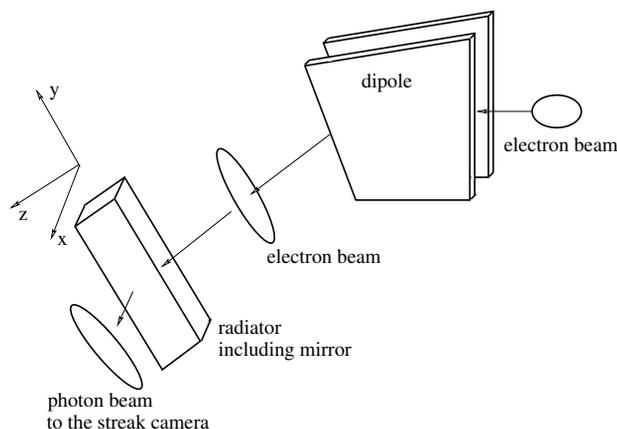
Figure 6: Setup for the measurement of the longitudinal phase space.
