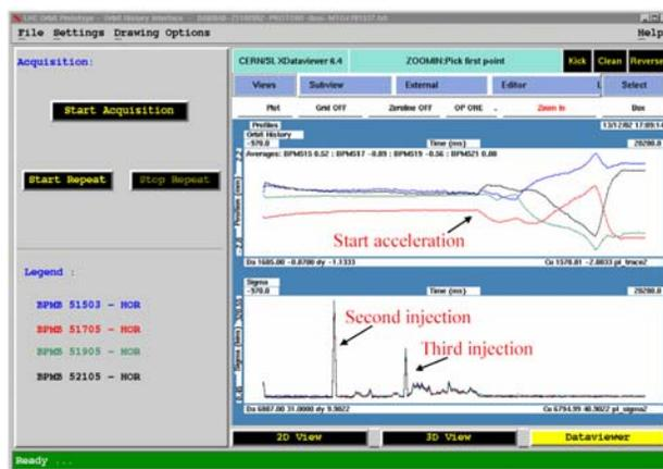
Figure 4. Control room display of the trajectory and orbit system during the 2002 tests on the SPS.
