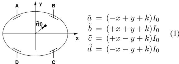
Figure 1: BPM Geometry and linear model equations
