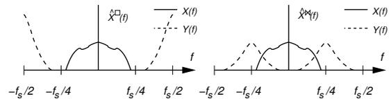
Figure 5: System frequency response (limited to the first Nyquist zone) showing  $y-x$  crosstalk for the “clockwise” (left) and “butterfly” (right) schemes.
