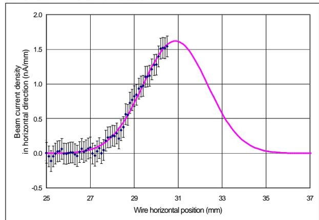
Fig. 1 Reconstructed horizontal profile of an electron beam with a current of about 10 nA. The reconstruction was done after a detailed noise analysis (see "noise studies").
