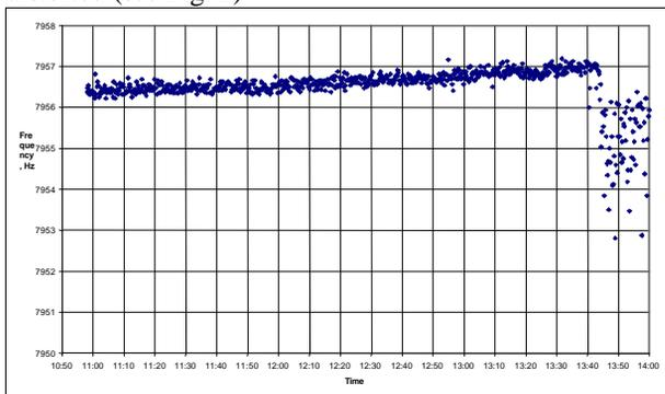
Fig. 2. Noise trace of the signal. At 13:43 the high frequency system was switched on and the noise appeared. Note that the beam was not present.
