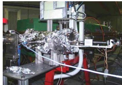
Figure 2: view of the FFC station installed on the Linac User port at 1GeV. The cable of the coaxial FFC is visible in the foreground. On the right hand side, there is the linear translation stage of the Stripline FFC.
