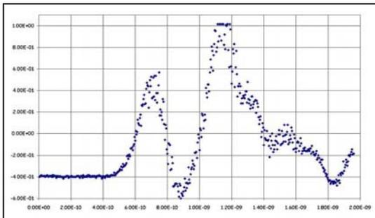
Figure 6: raw data from stripline FFC+Tek 5104. HOR: Eq. Time 200ps/div, VERT: 200mV/div. Two satellites are clearly visible.  $\Delta T$  is  $>330ps$  due to oscillatory pulse response.
