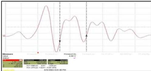
Fig. 5: Single Bunch acquisition, Coaxial FFC+Le Croy 8500 oscilloscope. HOR: RIS 200ps/div, VERT: 1V/div. At  $V_{phase}=3V$ , three 3GHz satellites can be observed.
