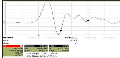
Fig. 7: Single Bunch: acquisition from Coaxial FFC+Le Croy 8500; HOR: RIS 200ps/div, VERT: 1V/div. At  $V_{phase}=2.7V$ , one main 3GHz satellite appears.
