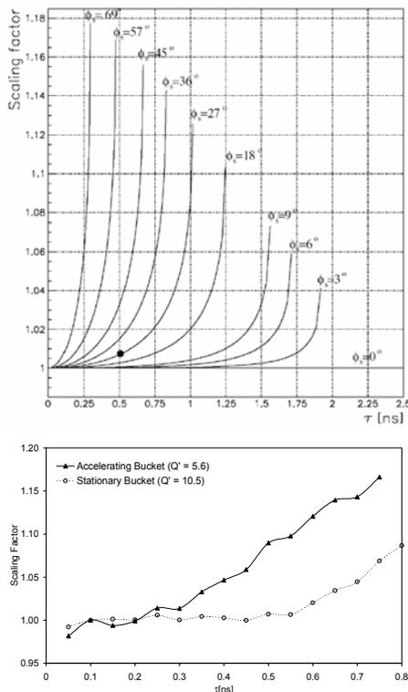
Figure 5. Scaling factor  $S_{sym}(\tau)$  as defined in Eq. 2 for a 200 MHz RF system and different values of the synchronous phase.
