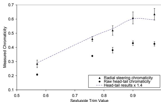
Figure 2. A comparison of head-tail and radial steering chromaticity, measured at 303GeV on the CERN-SPS.
