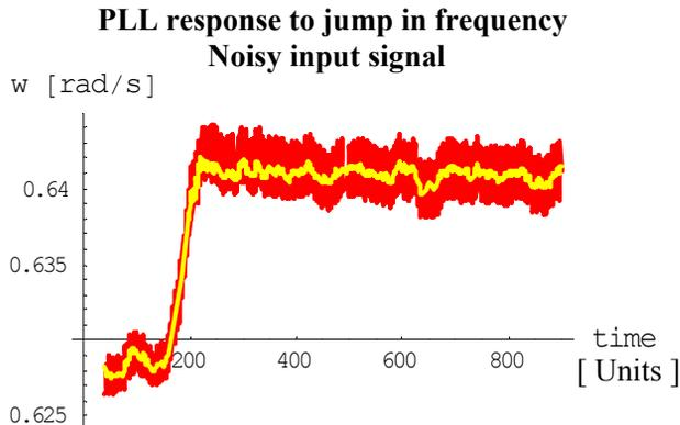
Fig 2. Red curve: Filtered PLL output.
