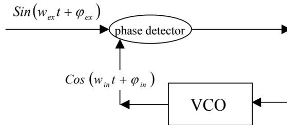
Often a PID regulation is added ( or in some cases, combined with the phase detector filter ), which allows locking on widely varying input frequencies:
