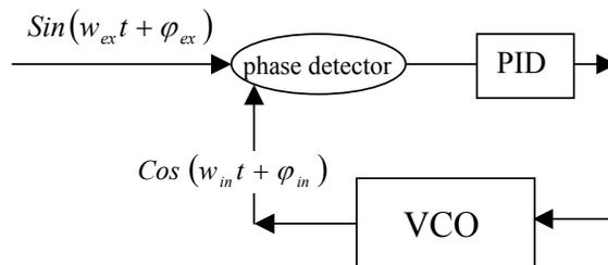
When the PLL is locked, the two inputs of the phase detector are 90 ° out of phase or “in quadrature”.
