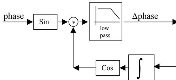
We can now introduce the concept of “phase detector” and VCO (Voltage controlled Oscillator):
