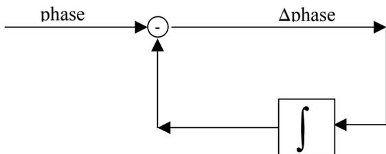
The definition of phase only has meaning when linked to a sine function. Since the sine function, which the PLL is locking on, is normally embedded within many other sine functions, only that phase should be extracted and the phases from the other sine function must be suppressed.
