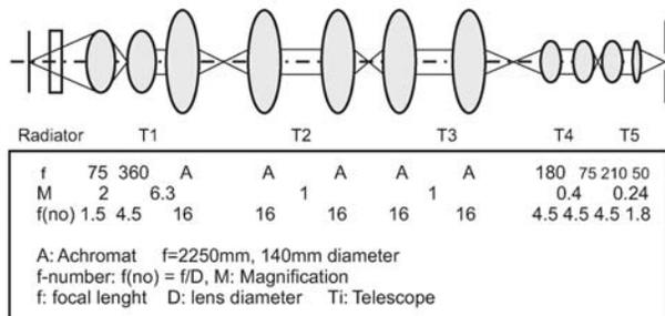
Fig. 5: Scheme of the full optical transmission line
