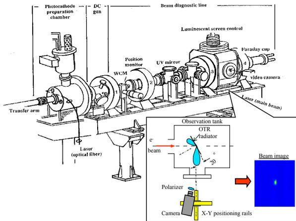
Figure 2: Layout of the electron beam line
