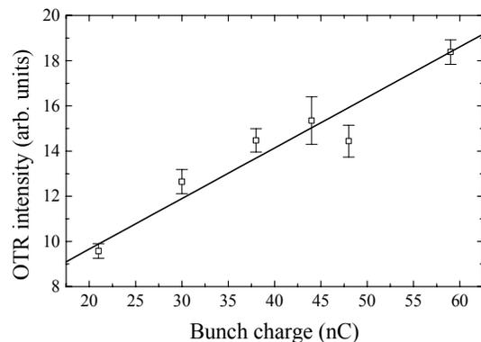
Figure 3: OTR light intensity versus the bunch charge.
