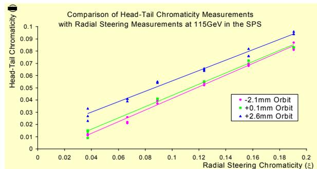
Figure 3: Head-tail versus classical  $Q'$  measurement [10]
