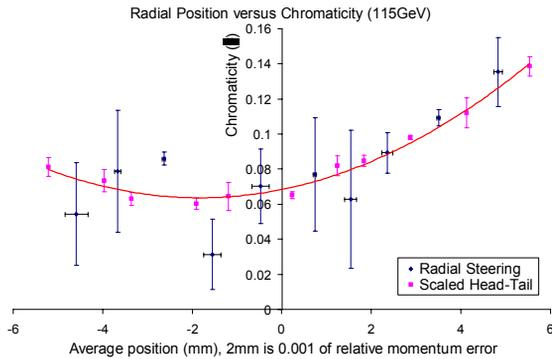
Figure 4: Non-linear chromaticity measured with head-tail oscillation [10]
