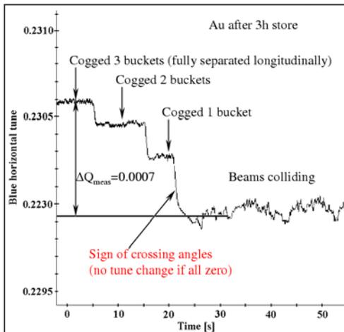
Figure 2: PLL-based beam-beam tune shift measurement at RHIC [7]
