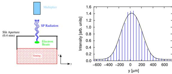
Figure 5: Left: Experimental arrangement for the horizontal SP beam monitor. Right: Measured horizontal intensity profile at observation angle  $\theta = 69.8^\circ$  corresponding to  $\lambda = 546$  nm,  $|n| = 1$ . Dashed line: best fit supposing a normal distributed beam profile and a rectangular distribution function for the aperture resolution.
