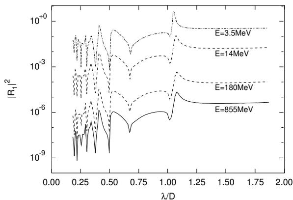
Figure 2: Calculated functional dependence of the radiation factor  $|R_1|^2$  on the normalized wavelength  $\lambda/D$  according to Ref. [23] for a grating with  $\alpha_{blaze} = 41.12^\circ$  as used in Ref. [19]. The quoted beam energies correspond to the different accelerator sections of the Mainz Microtron MAMI.
