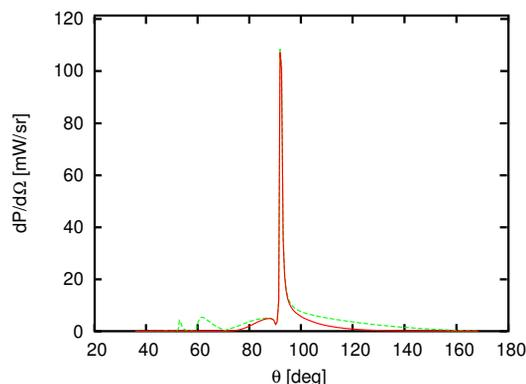
Figure 4: Emittted power in first order as function of angle of observation taking into account the angular dependency of  $|R_1|^2$  for the échelette grating of Fig. 2.
