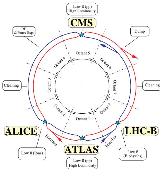
Figure 1: Layout of LHC ring and experiments.
