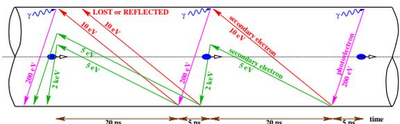
Figure 10: Principle of electron cloud buildup.
