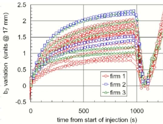
Figure 2: Injection drift of the sextupole field component for a sample of LHC main dipoles due to the decay of the persistent currents [3].  $\Delta b_3 = 1$  unit corresponds to  $\Delta Q' = 50$  units. The persistent currents 'snapback' to their value before injection during the first seconds of the energy ramp (time = 1000 s).
