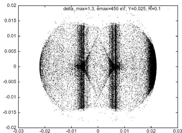
Figure 11: Simulated transverse distributions of electrons due to multi-pacting in the LHC vacuum chamber [1].
