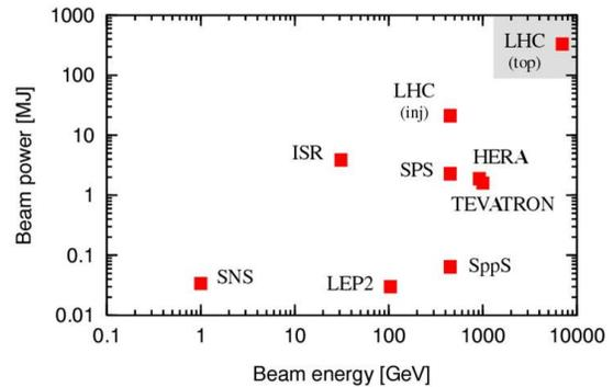
Figure 6: Energy stored in various accelerators.
