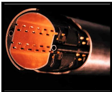
Figure 9: The LHC vacuum chamber and the beam screen (at 4 – 20 K) that shields the cold mass from synchrotron radiation and image currents. In this figure the chamber is rotated by  $90^\circ$  with respect to its normal orientation.
