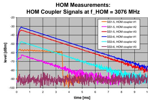
Figure 5: HOM-coupler signals of a high-Q mode.
