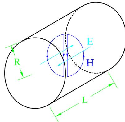
Figure 1: Cylindrical “pill-box” cavity, shown with the field lines of the  $\text{TM}_{110}$  dipole mode (horizontal polarized).
