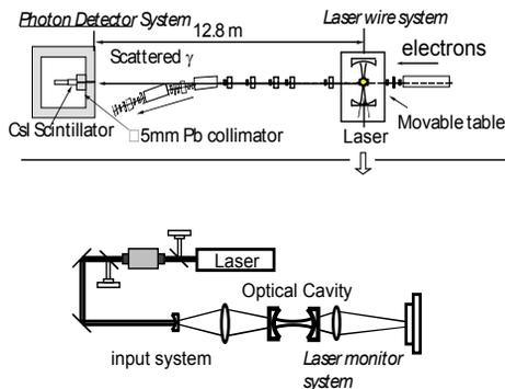
Figure 1: ATF CW laser-based profile monitor schematic.
