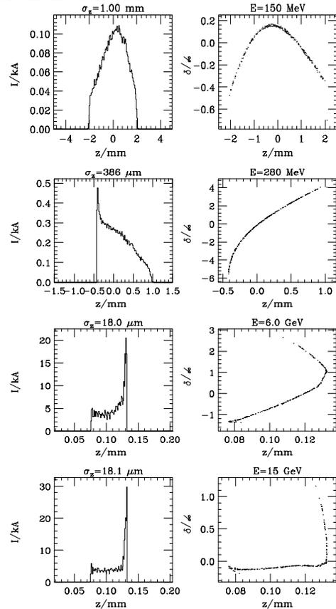
Figure 4: Evolution of longitudinal phase space in the LCLS. The plots show the  $z$  distribution and the  $E - z$  correlation following (from top to bottom): a) the gun capture section, b) the first compressor section, c) the second compressor and d) at the end of the linac.
