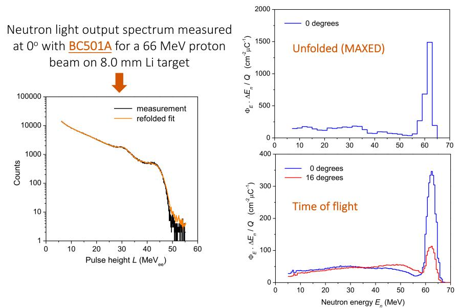
Time of flight measurement of neutrons produced by a 66 MeV proton beam irradiating an 8.0 mm <sup>nat</sup>Li target. (<u>EJ-276</u> at 8.00 m from the target at 16°).
