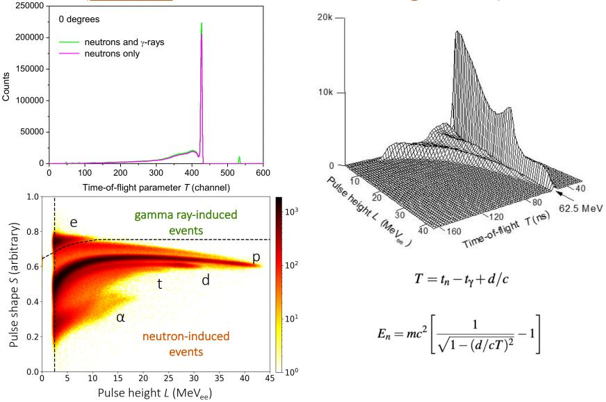
Measured light output spectra for neutron energies between 10 - 65 MeV, selected by time-of-flight for <u>BC501A</u>.
