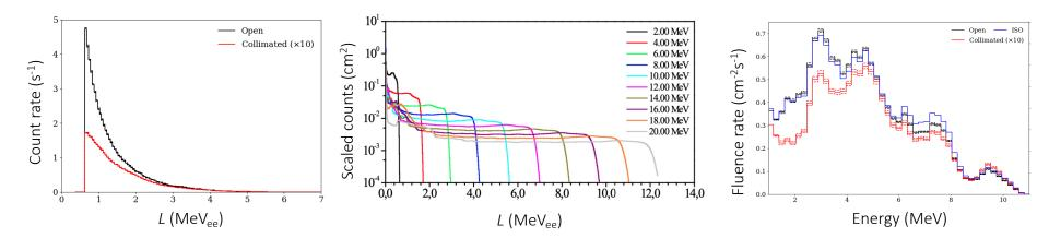
Measured neutron pulse height spectrum ...
