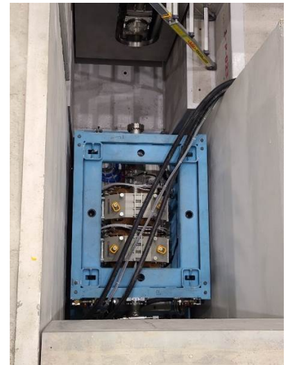
Final focusing & wobbler module in ISOL bunker
