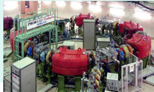
Each of the three gantries is three-story weighs 200
