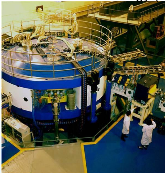
CYCIAE-100 High current Proton Cyclotron Current: 200 \mu A
