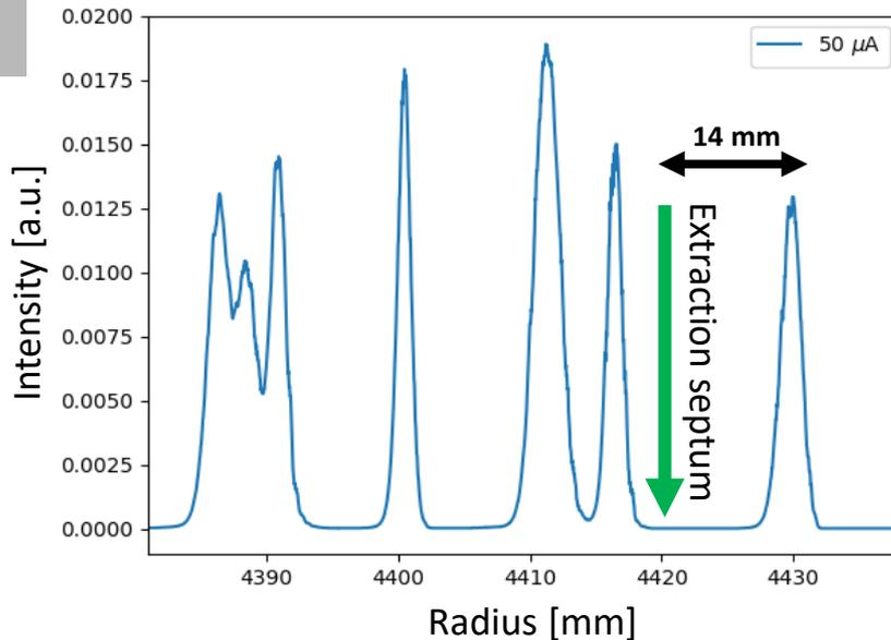
Radial probe measurement at the extraction of the PSI 590 MeV cyclotron (June 2021):
