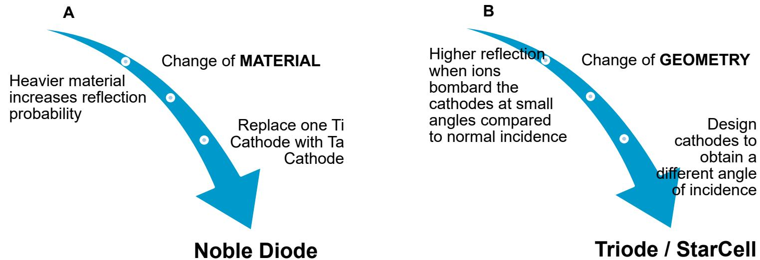
Both solutions do improve the pumping speed and stability for noble gases
