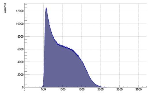
Pulse height spectrum of plastic scintillator
