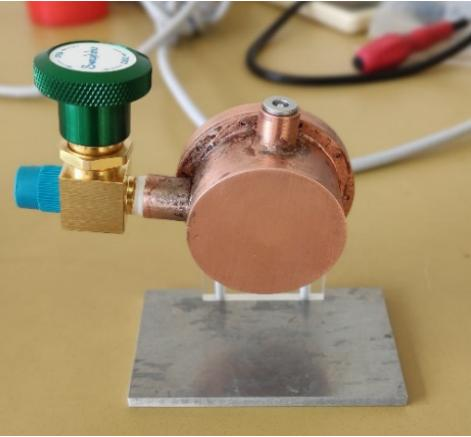
Assembly of fission chamber assembly
