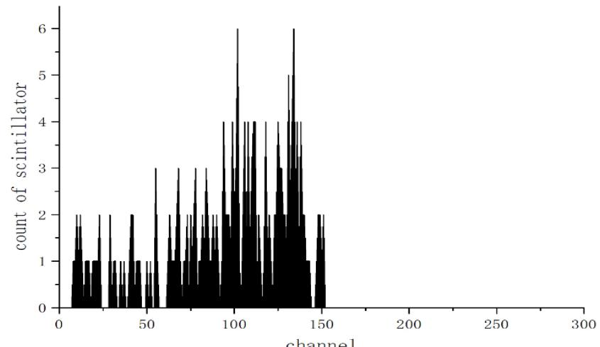
Coincidence events pulse height spectrum for silicon
