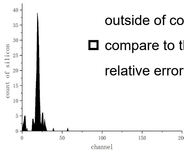
Coincidence events pulse height spectrum for silicon
