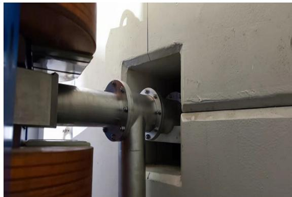
Proton vacuum beam pipe
