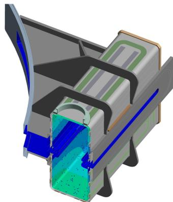
New cavity body heat flux map for a 140-kW dissipated power
