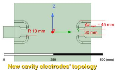
New cavity electrodes' topology
