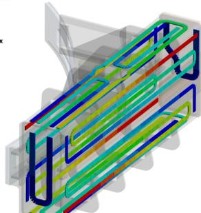
Water temperature in cooling channels
