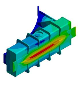
New cavity deformation
