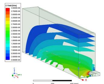
3D electric field for a 700-kV cavity voltage
