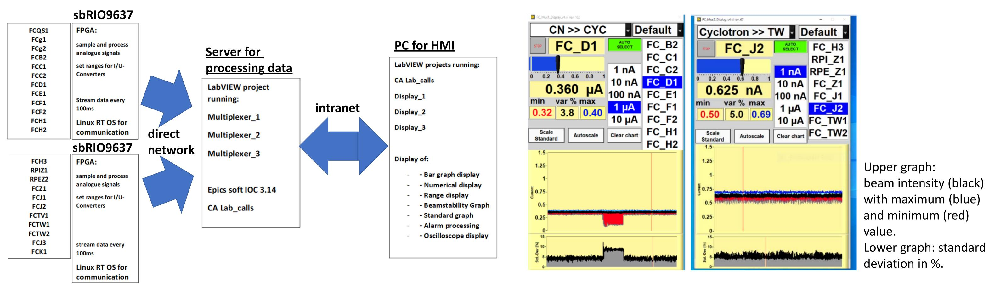
New setup: 30 channels for Faraday cups are connected to two PCB's interfacing between I/U-converters and 2 boards of NI-sbRIO9637. These boards process analogue values with 10kHz and stream every 100 ms the data to the server, where these data are processed and published to the intranet via the EPICS softIOC.
