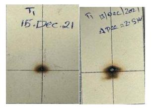
Here we see a paper burn test, which show the beam location and profile when it hit the target
