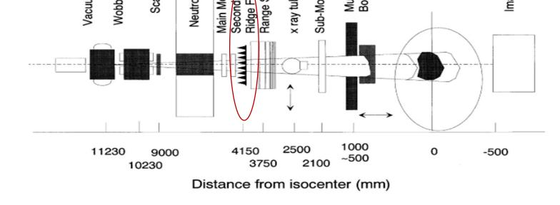
• The Bragg peak of the single energy particle beam is broadened to a flat dose distribution region by the modulator's geometry and relative motion.
