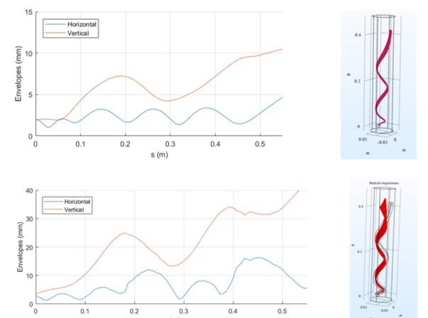
Figure 6: Envelope simulation considering space charge. The upper plot shows the simulation with 1 nA injection beam. The lower one shows that of the 10 mA injection beam. The frame of a spiral pipe in the lower 3D beam plot shows the reference beam path without considering the space charge effect. The reference orbit is changed by the space charge. A further design study of a shielding structure is needed to remove the repulsive force from different turns.
