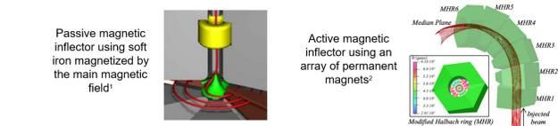
Figure 1: Two types of magnetic inflector.
