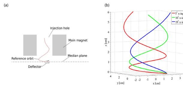
Figure 2: Reference orbit in the injection hole. (a) shows the conceptual model. By tracking the particle reversely from the median plane to the injection point with different Pitch angles, the different reference orbits are shown in (b).
