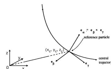
Figure 3: The moving optical coordinate system.
