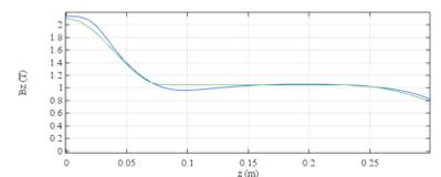
Figure 5: On-axis magnetic field in the injection hole after optimizing the shape of the center plug. The green line is the objective field that could properly focus the beam in the inflector. The blue line is the on-axis magnetic field produced by the designed main magnet with a properly shimmed central plug.
