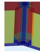
Figure 4: Steel plug in the injection hole. Blue colored structure is the vacuum region. Green is the sector pole. Red is the solid steel structure in the injection hole.
