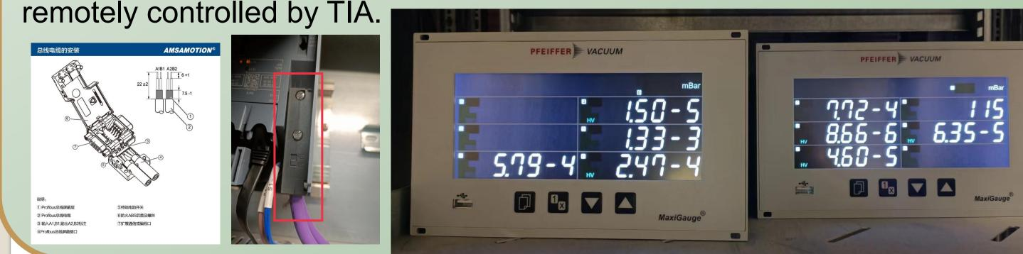
The right figure shows the Human Machine Interface (HMI) of the vacuum control and interlocking system of the beam line based on PLC.
