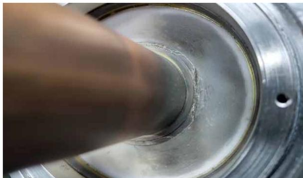
Figure 4: RF window coated with silver brazing solder.
