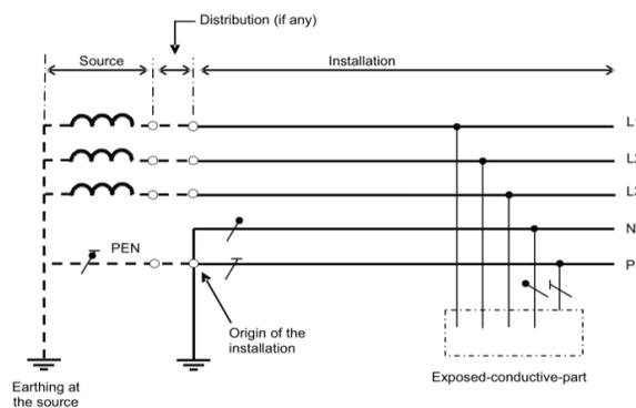
Figure 3: TN-C-S system 3-phase, 4-wire, where the PEN is separated into PE and N at the origin of the installation [7].
