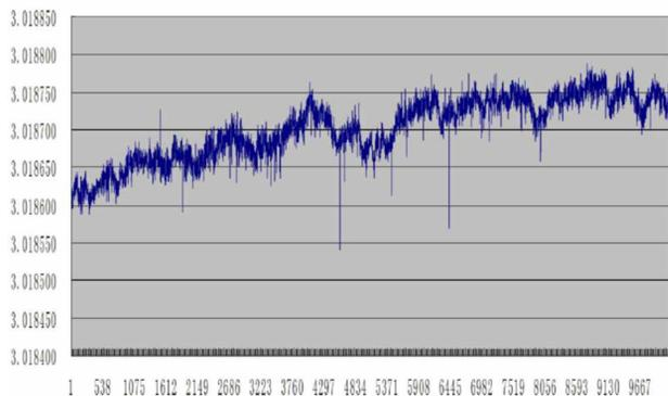
Figure 2: Current instability test of main magnet power supply in long term operation (8 h).
