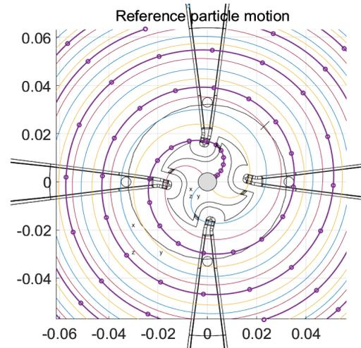
Figure 7: Four trajectories of reference particles are shown. Dots mark every 180 RF degrees.
