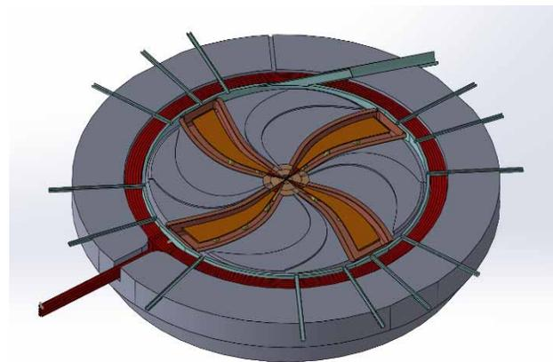
Figure 2: Parametrized model of the cyclotron.
