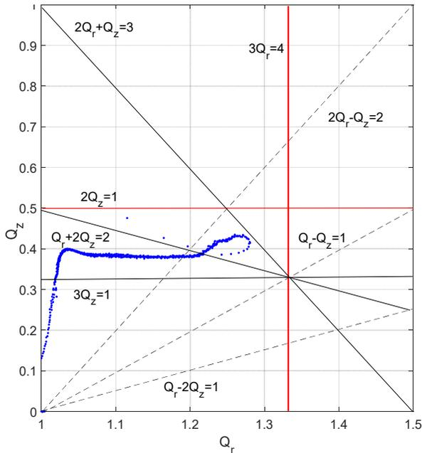
Figure 3: Tune diagram.
