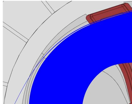
Figure 10: The beam tracing in the cyclotron structure.
