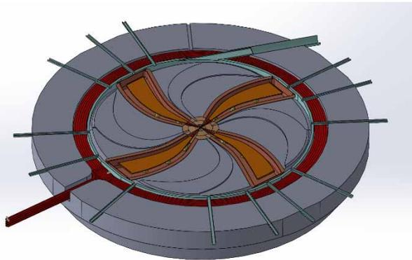
Figure 1: 3D computer model of the cyclotron.
