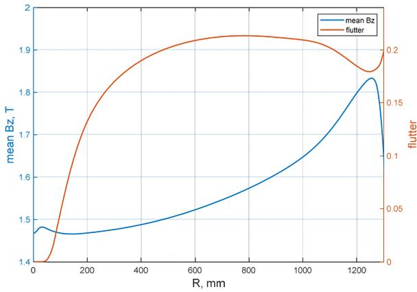
Figure 2: Average magnetic field and flutter along the radius.
