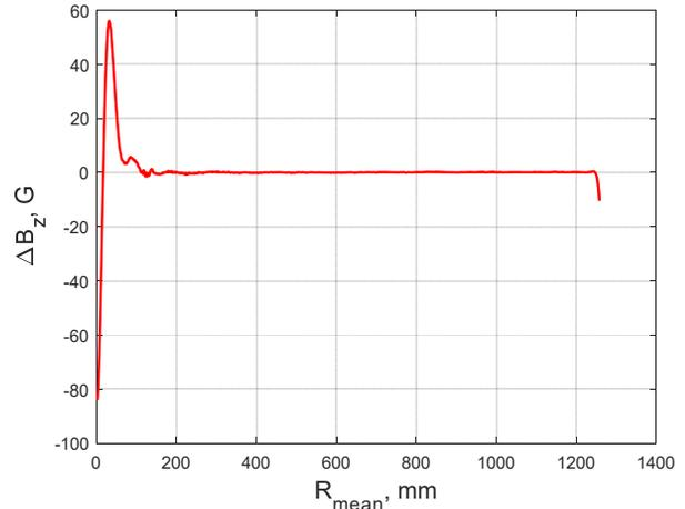
Figure 5: Difference between average magnetic field and isochronous one.
