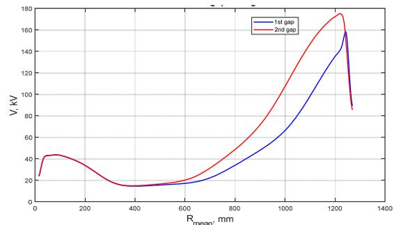
Figure 7: Voltage distribution along radius.
