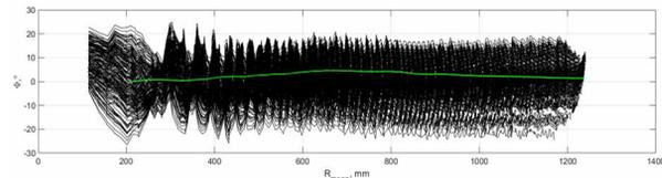
Figure 9: Integral phase slip along the radius. Positive phase corresponds to the lagging particle. Black lines – phase motion of the beam from particle tracking, green line – CORD.
