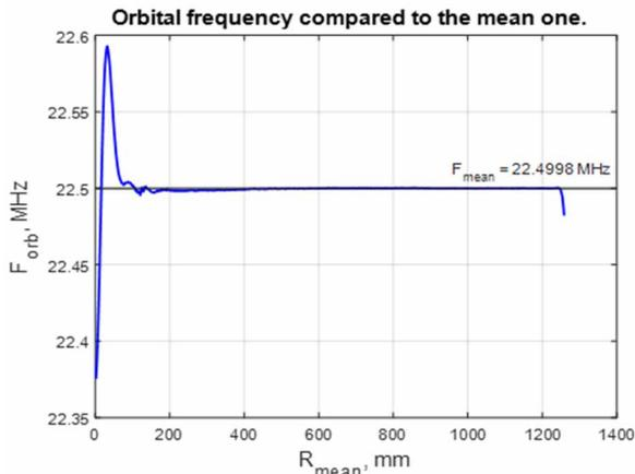
Figure 4: Orbital frequency against radius.
