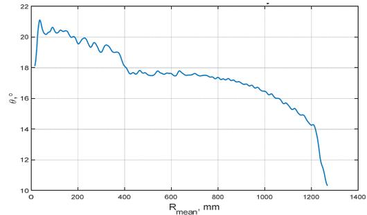
Figure 6: Azimuthal extent of the cavities against radius.
