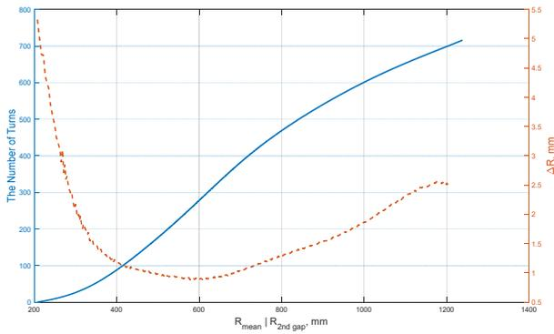
Figure 8: Number of turns (blue solid line) and orbit separation distance (red dash line) in the cyclotron along the radius.
