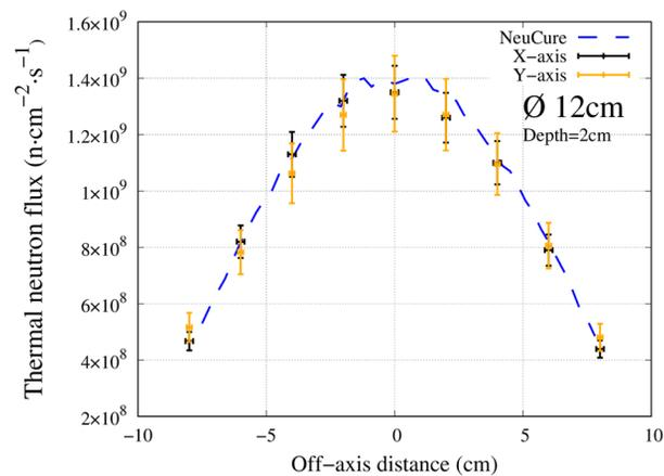
Figure 3. Off-axis thermal neutron distribution inside the water phantom at a depth of 2 cm for the 12 cm diameter collimator.
