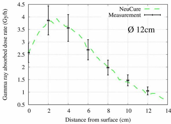
Figure 5. Gamma ray dose rate distribution along the beam central axis for the 12 cm diameter collimator.
