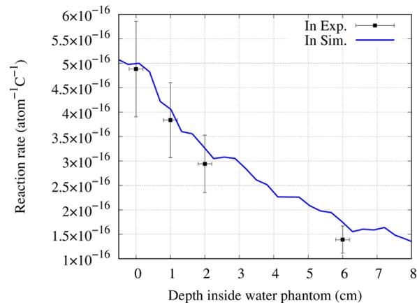
Figure 4. Fast neutron distribution along the beam central axis for the 15 cm diameter collimator.
