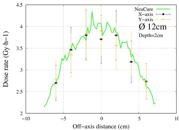
Figure 6. Off-axis gamma ray dose rate at a depth of 2 cm inside the water phantom for the 12 cm diameter collimator.
