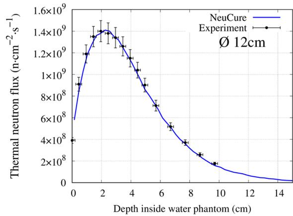
Figure 2. Thermal neutron distribution inside the water phantom along the beam central axis for the 12 cm diameter collimator.
