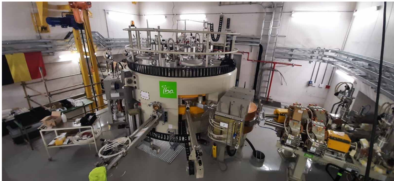
Figure 3: The C70 cyclotron installed in its final position.
