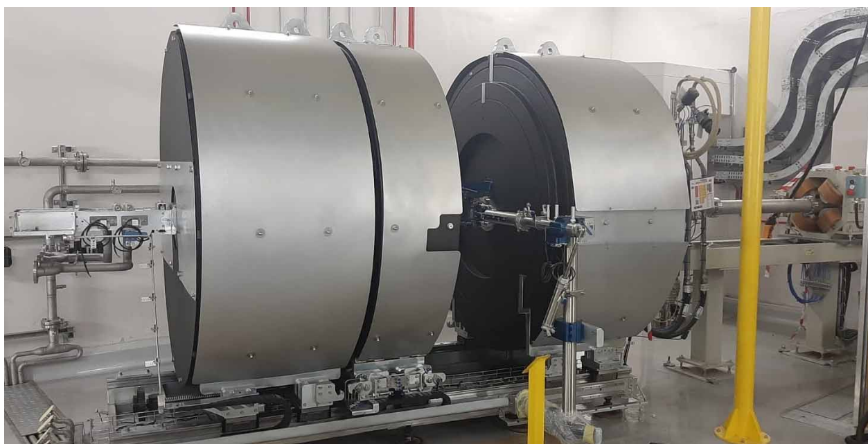
Figure 6: The SAIF target station showing the pneumatically controlled pusher arm and robot arm mechanisms.
