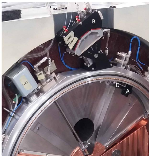
Figure 7: Extraction system and diagnostics: (A) Stripper carousel, (B) target changer, (C) pop-up probe and (D) left/right collimators through the vacuum chamber.
