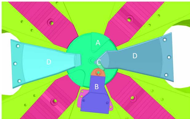
Figure 4: Central region: (A) central plug with iron extensions, (B) Ion source, (C) puller and (D) dee tips.
