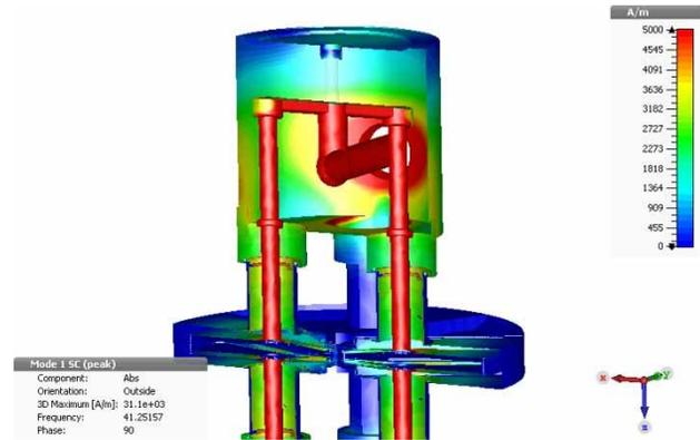
Figure 5: Surface current distribution in the RF cavity.
