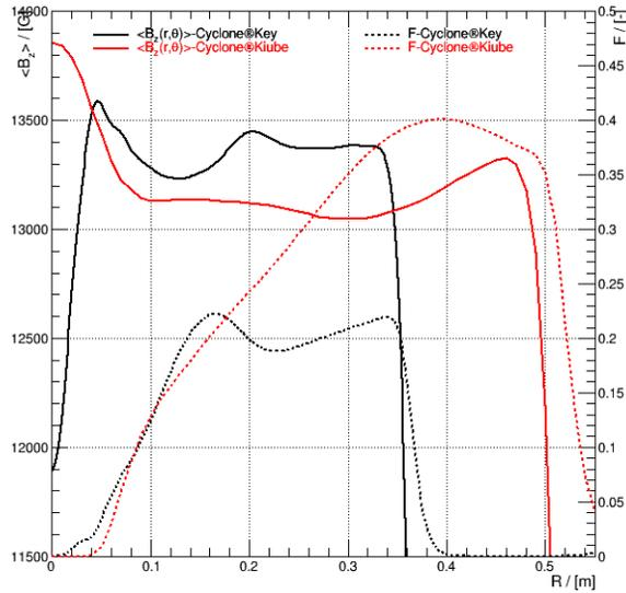
Figure 3: Average magnetic field and flutter in the Cyclone® KEY and in the Cyclone® KIUBE.
