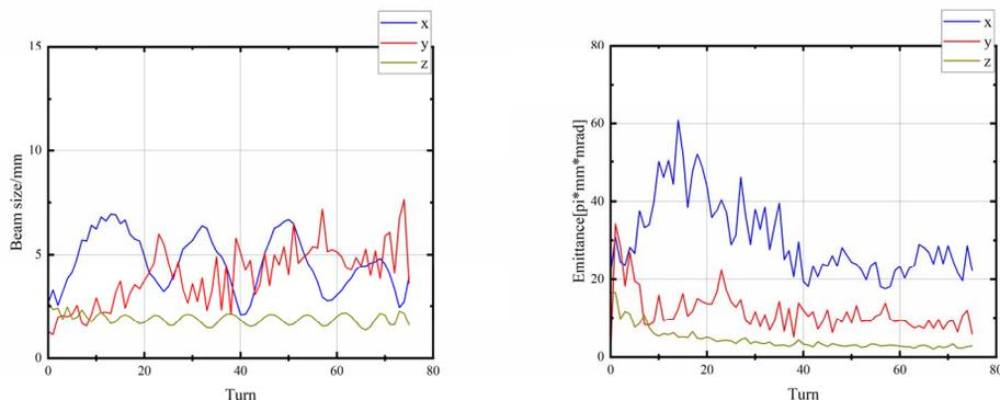
Figure 7: RMS Beam size(left) and RMS Geometry Emittance(right). The RMS beam size of last turn in x, y and z is 3.91555, 3.60329 and 1.58493mm; The RMS geometry emittance of last turn in x, y and z is 22.27046, 5.83704 and 2.77792 pi•mm•mrad.
