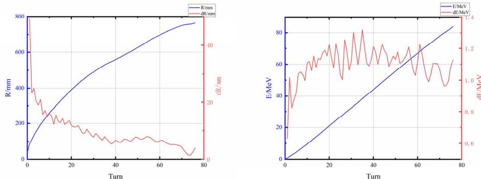
Figure 6: Turn separation(left) and Energy gain(right). The last turn separation could reach 5mm, and the energy gain per turn is about 1.2 MeV.
