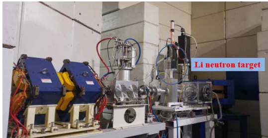
Figure 4: Quasi-monoenergetic neutron source.
