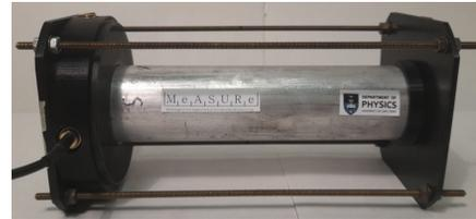
Figure 3: The compact spectrometer comprised of an EJ-276 scintillator optically coupled to a silicon photomultiplier, with an aluminium and 3D printed casing.
