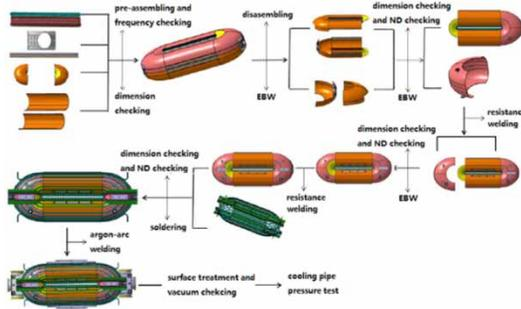
Figure 7: Cavity's mechanical fabrication process.
