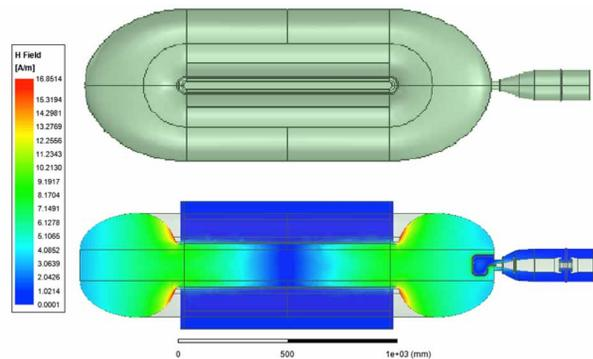
Figure 1: RF design of the cavity and coupler.
