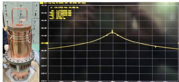
Figure 11: Cavity coupler and Q measurement.
