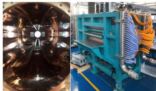
Figure 10: Cavity inside and the cavity assembly at the installation site of CIAE.
