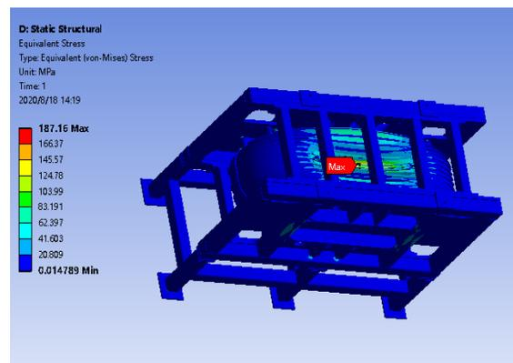
Figure 6: Stress for +176 kHz frequency tuning.
