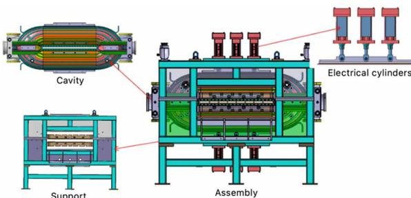
Figure 3: SolidWorks model of the cavity assembly.
