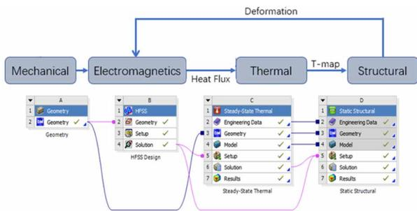
Figure 2: Workflow and ANSYS Project Schematic.
