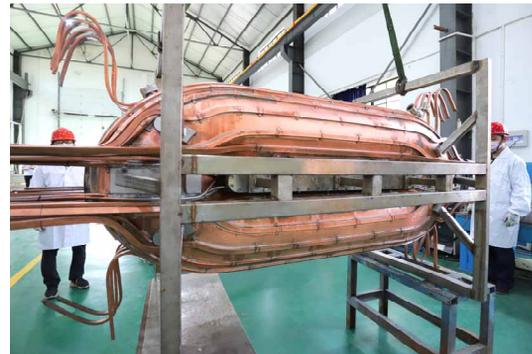
Figure 9: Cavity outside look after the soldering of all the cooling pipes.
