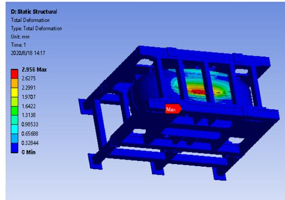
Figure 5: Deformation for +176 kHz frequency tuning.
