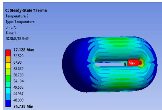
Figure 4: Temperature distribution on the cavity walls.
