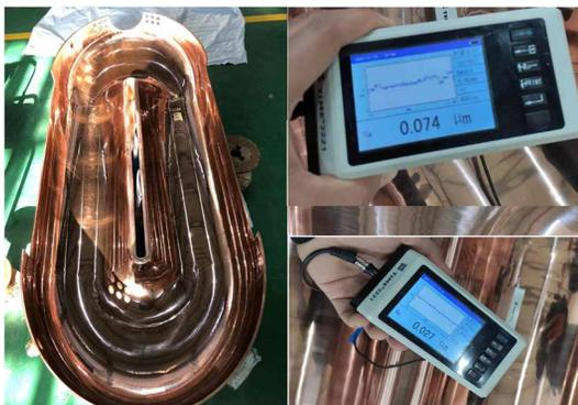
Figure 8: One of the two half-cavities and the surface roughness measurement.
