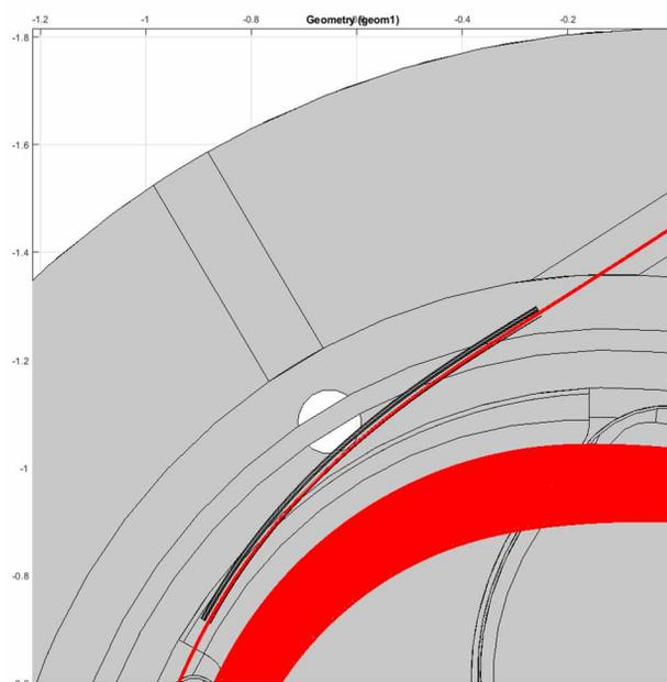
Figure 6: The beam tracing in the cyclotron structure.
