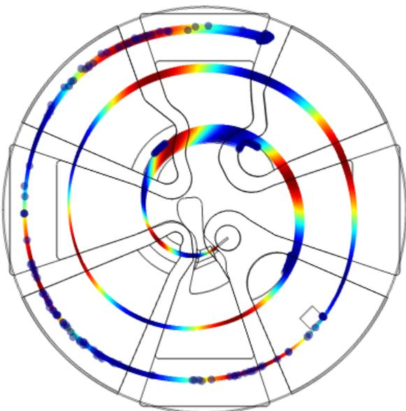
Figure 5: Beam trajectories in the optimized center (Comsol). Color indicates oscillation phase of the accelerating system.
