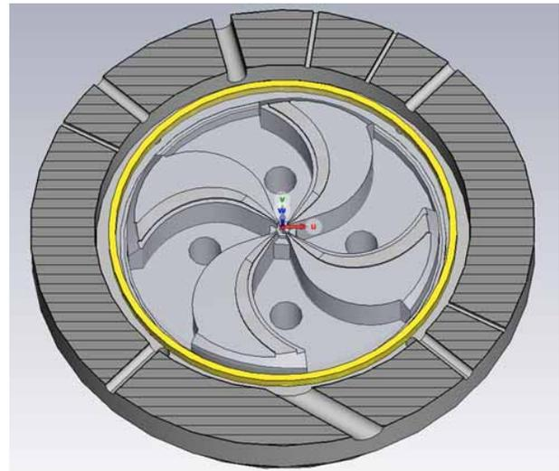
Figure 3: Magnet of the cyclotron MSC230.
