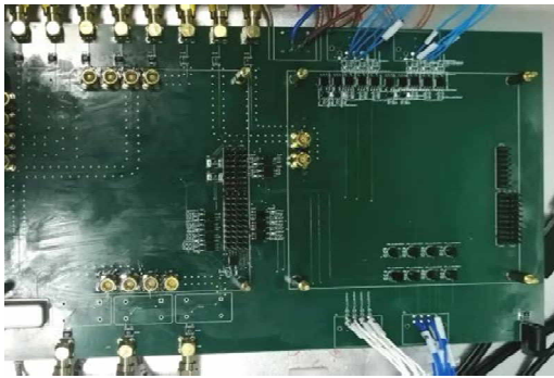
Figure 3: Motherboard for LLRF system board.
