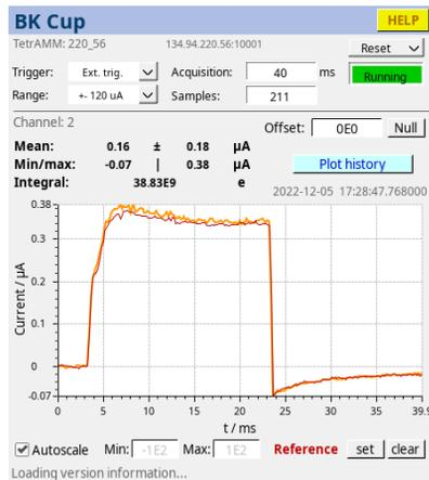
Figure 8: Beam current measurement at BigKarl Cup showing a pulsed beam of  $\sim 40$ nA.
