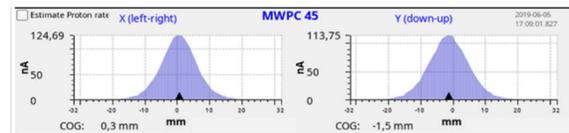
Figure 6: Beam profile at Big Karl target station. The beam size shown is ~15 mm FWHM.
