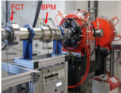
Figure 7: Beamline inside Big Karl area with Beam Position Monitor System (BPM) and Fast Current Transformer (FCT).
