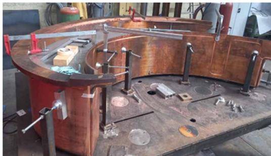
Figure 8: Shop test assembly of a C400 liner.
