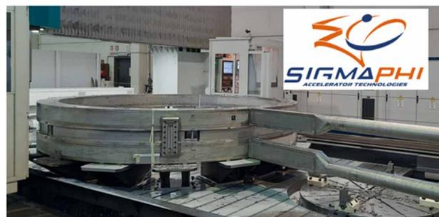
Figure 6: C400 Helium vessel, welding completed.
