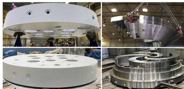
Figure 5: Manufactured part of C400 yoke.
