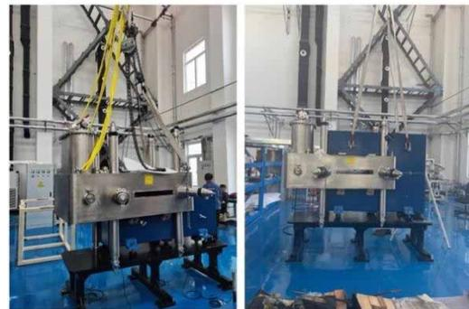
Figure 11: 1:4 scaled magnet assembly.
