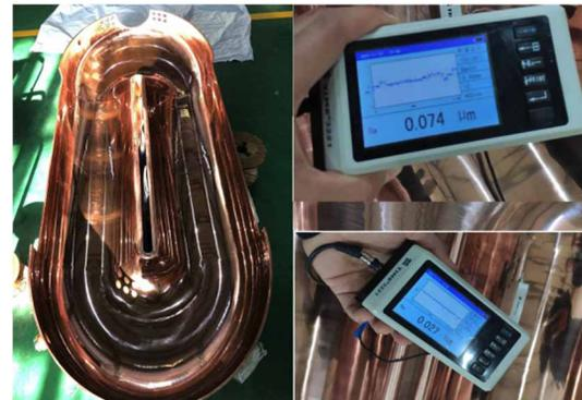
Figure 15: One of the two half-cavities and the surface roughness measurement.
