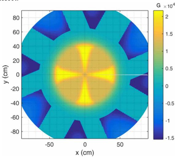
Figure 2: Axial magnetic field distribution in the middle plane.
