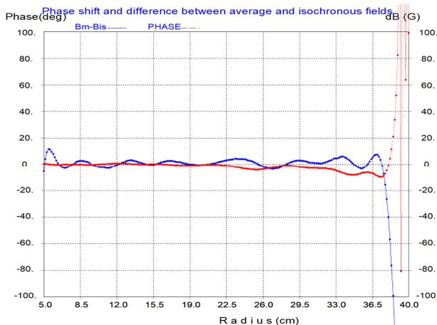
Figure 3: The deviation of the average field from the isochronous field and the slip phase.
