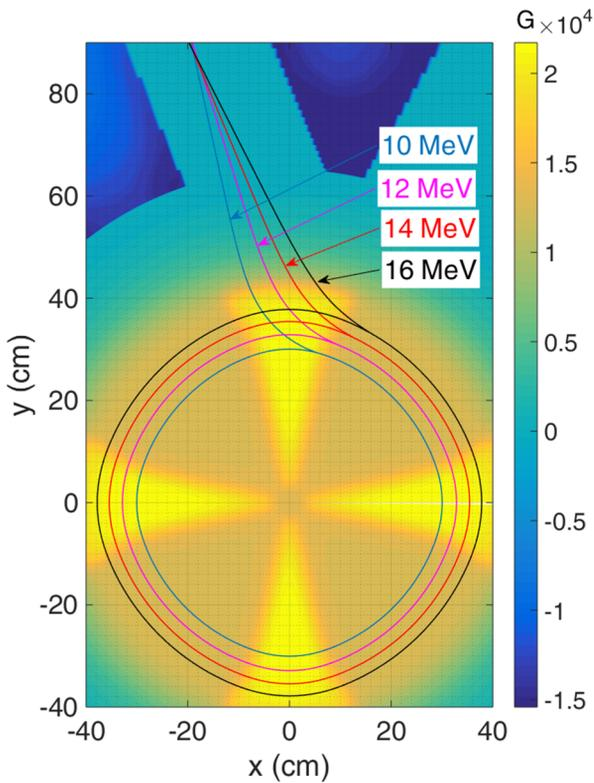
Figure 5: Extraction trajectories of particles with different energies.
