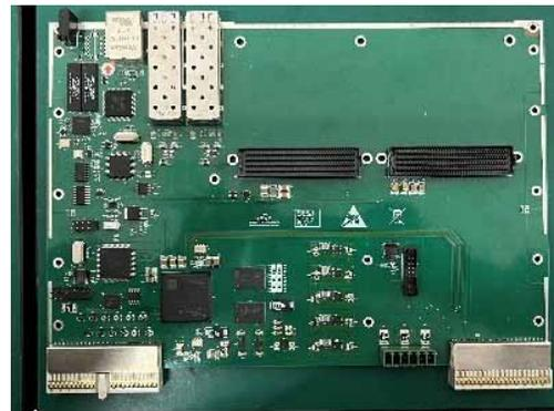
Figure 5: the vertical deflector controller motherboard.
