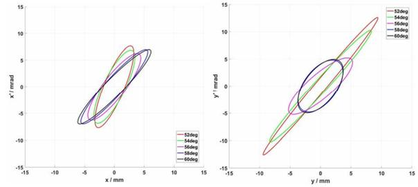
Figure 4: The horizontal (left) and vertical (right) distributions with different azimuths of the stripping foil at the entrance of the beam line.
