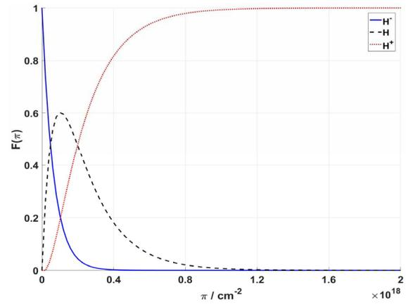
Figure 6: Fractions of hydrogen beam with different thickness of the carbon foil.
