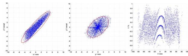
Figure 3: The particle distribution at the entrance of the beam line in horizontal (left), vertical (middle) and longitudinal (right) phase space.
