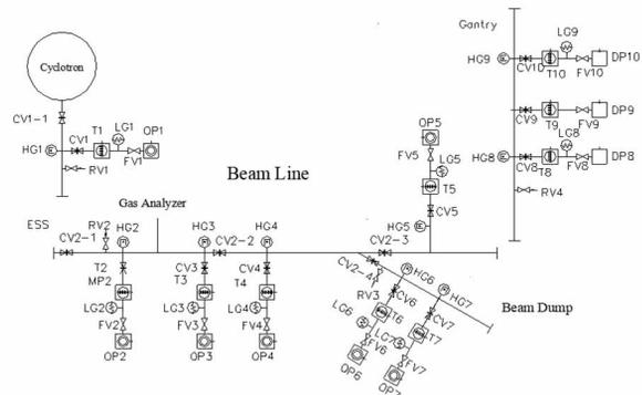
Figure 2: Layout of beam line vacuum system.
