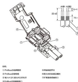
Figure 4: The wiring diagram of the Siemens DP connector.
