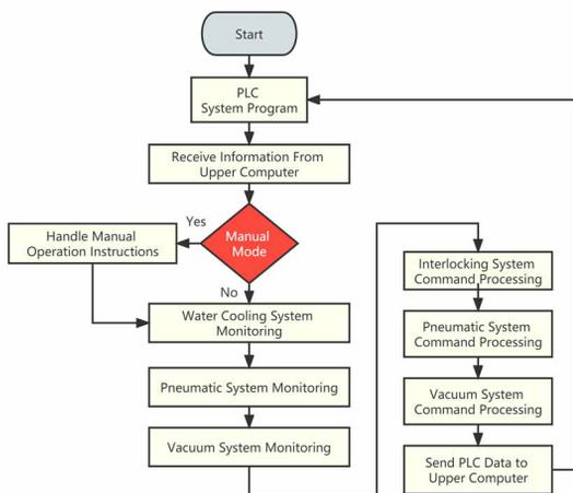
Figure 7: The flow chart of the PLC program.
