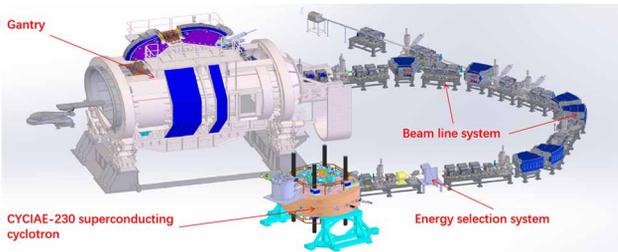
Figure 1: Layout of CYCIAE-230 and beam line.
