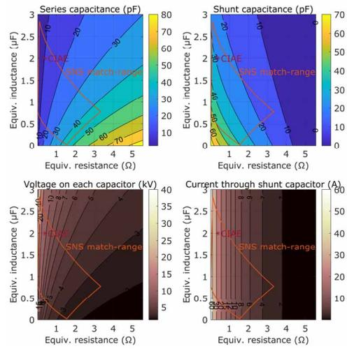
Figure 6: Electrical requirement contours for the type- $\gamma$  network for the 500 W 13.56 MHz chain.
