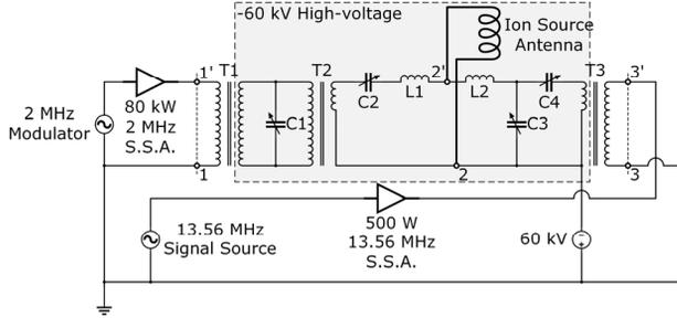
Figure 4: Design of the matching structure.
