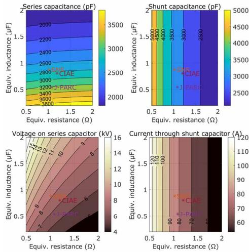
Figure 5: Electrical requirement contours of the series and shunt capacitors in the type-L matching network with 3:1 transformer for the 80 kW 2 MHz chain. Impedances of projects marked by coloured stars.
