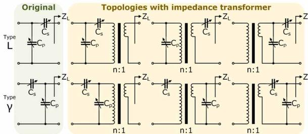
Figure 3: Dual-capacitor type-L and - $\gamma$  matching networks with or without an impedance transformer.  $C_s$  stands for the series capacitor and  $C_p$  stands for the shunt one.
