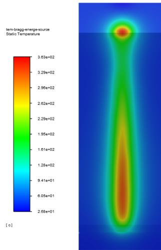
Figure 9: Temperature Distribution of the Electron Beam Size is 10 mm.
