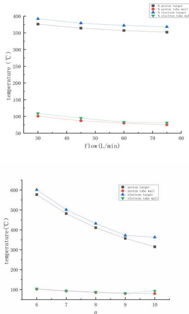
Figure 8: Curves of the Maximum Temperature, (a) different flow rate at beam size 9 mm, (a) different beam size at flow rate 1 kg/s.
