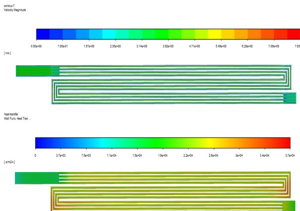
Figure 4: Distribution of Velocity and Convective Heat Transfer Coefficient.
