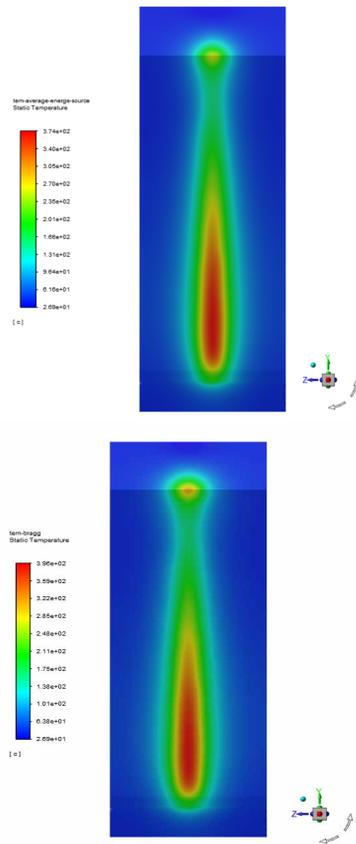
Figure 7: Temperature distribution of average density in depth direction, (a) target stopping 100 MeV proton, (b) target stopping 5 MeV electron.
