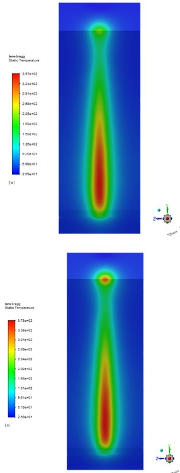
Figure 6: Temperature distribution of calculation energy probability density in depth direction by FLUKA, (a) target stopping 100 MeV proton, (b) target stopping 5 MeV electron.
