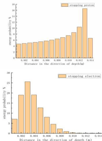
Figure 2: Energy probability in the beam dump of (a) 100 MeV proton, (b) 5 MeV electron.
