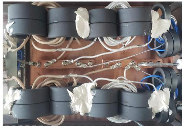
Figure 4: Transmission line transformer.
